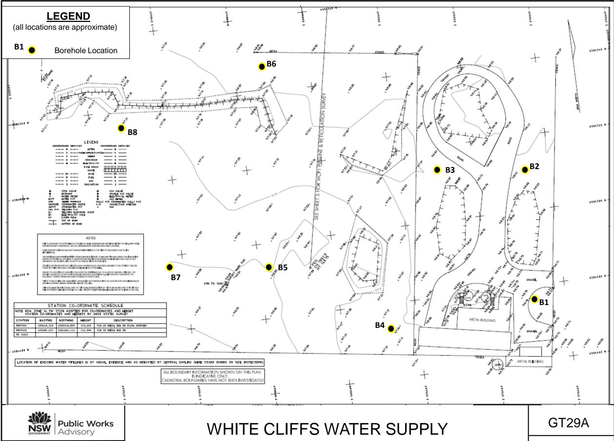
Borehole Location Plan - Water Treatment Plant
