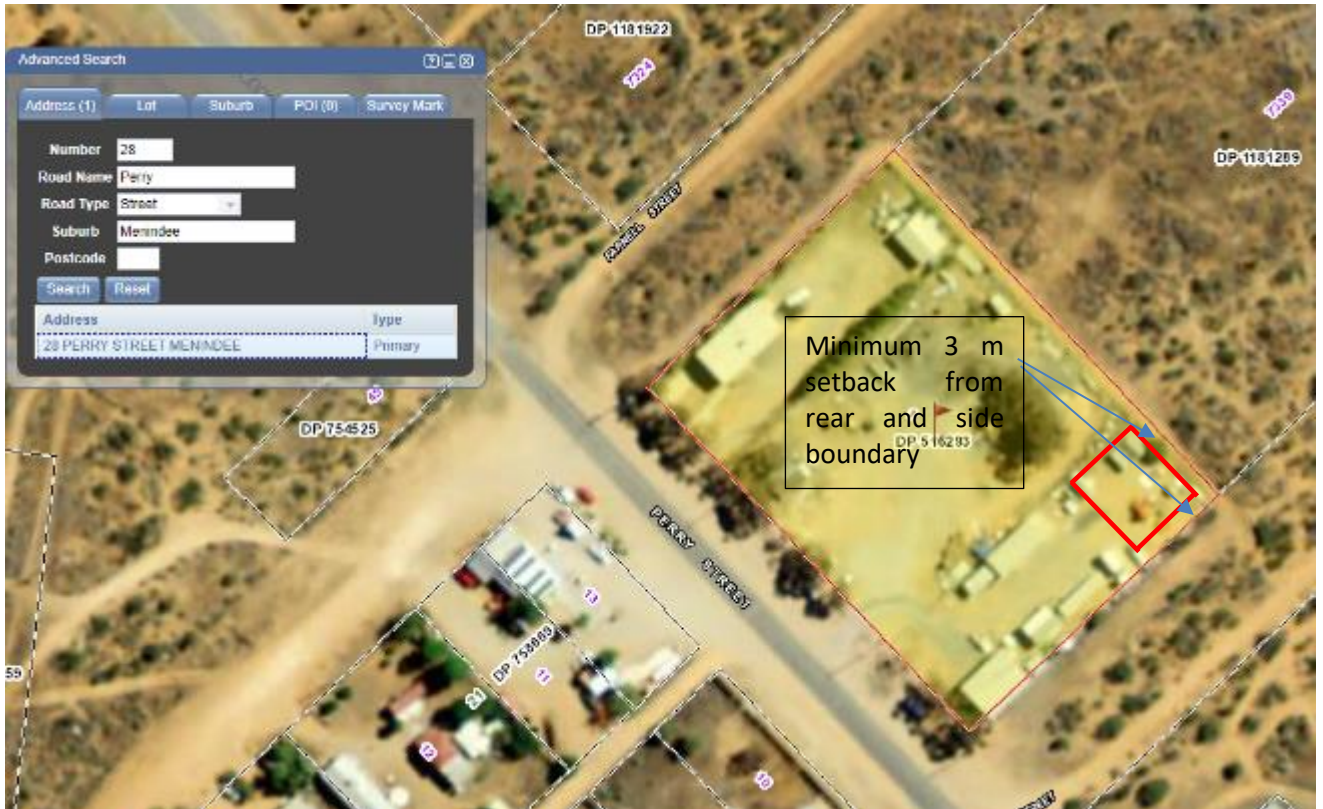
Photo 1: Site location plan of shed at Menindee works depot - shed dimensions are 16m by 12m. (source 6 maps)
