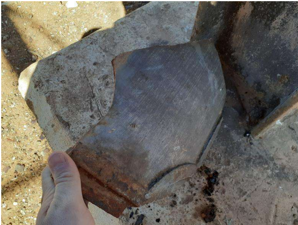
Figure 9 - Example of Cast Iron piece, having already broken away from the rest of the rest of the tank
