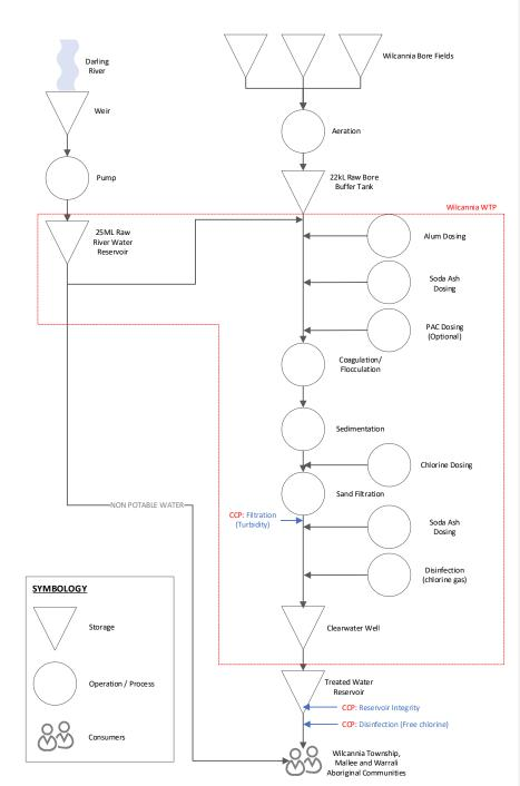
Figure 2 Wilcannia DWSS Process Flow Diagram
