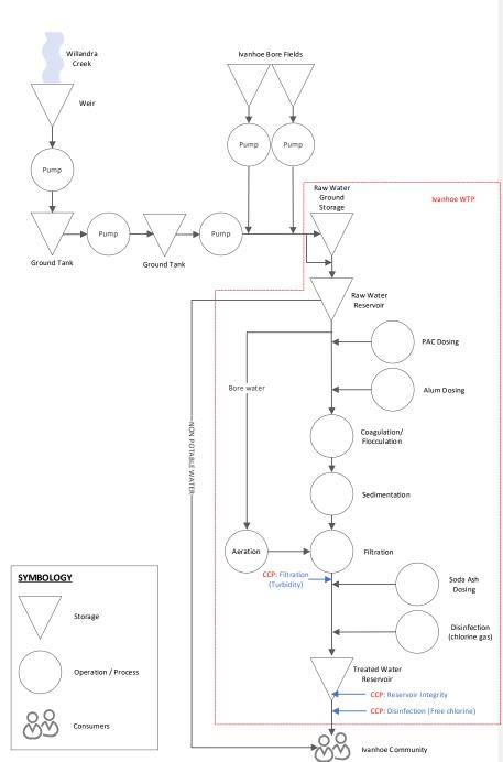
Figure 3 Ivanhoe DWSS Process Flow Diagram
