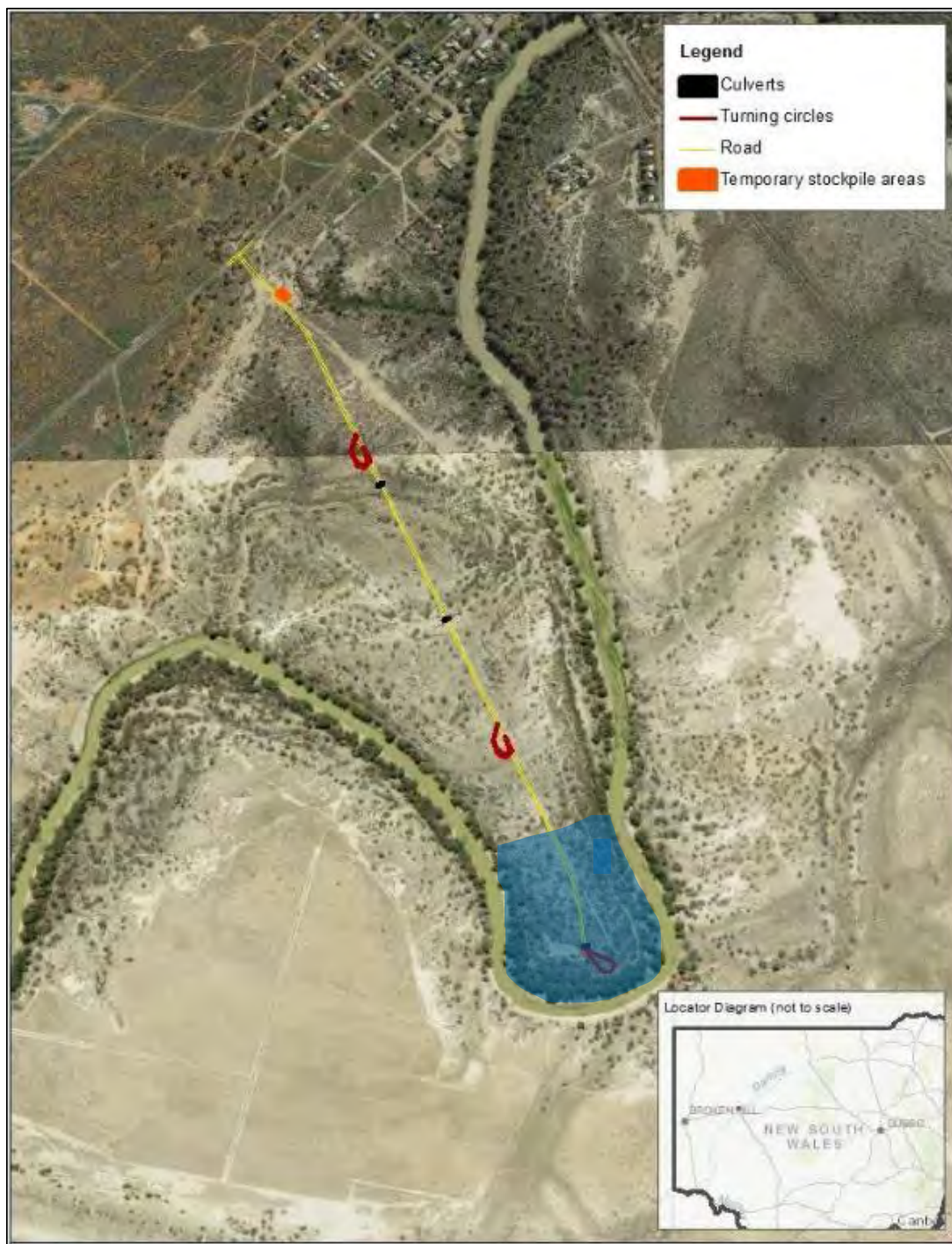
Figure 9: Union Bend Reserve – new access road plan (Union Bend Reserve highlighted in blue) (Source: Water NSW REF 2021)
