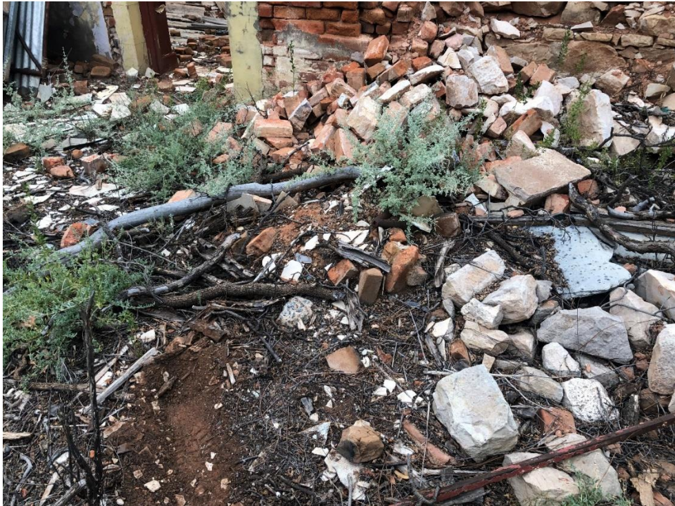
Figure 6.4: Fragments of fibre cement among building rubble.
