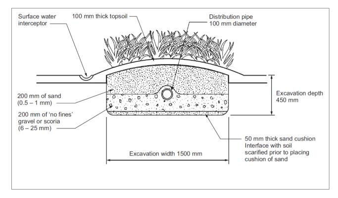
NOTE: An LPED line can be used to dose load the ETA/ETS bed.
