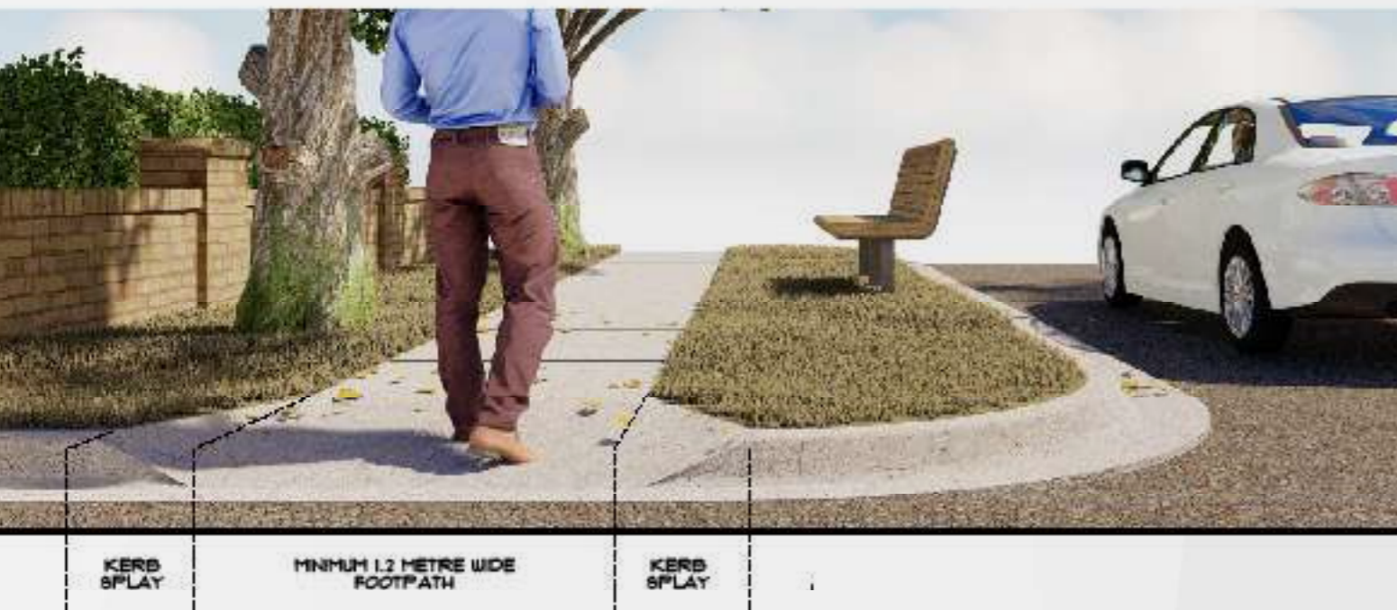
Typical Compliant Kerb Ramp Arrangement
