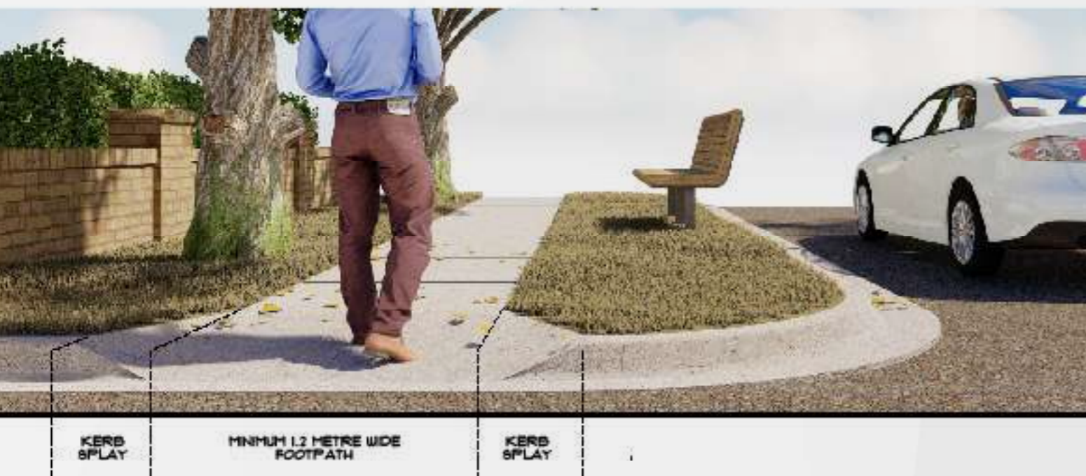
Typical Compliant Kerb Ramp Arrangement
