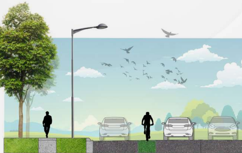
Road Reserve | Footpath 1.2m | Road Reserve | Parking Lane | Cycle Lane | Travel Lane | Travel Lane
