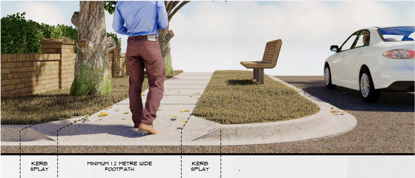
Typical Compliant Kerb Ramp Arrangement
