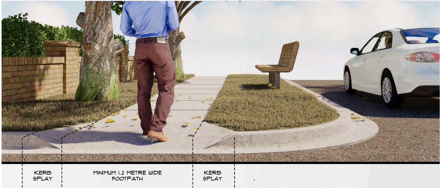
Typical Compliant Kerb Ramp Arrangement
